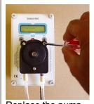
Replace the pump cover and the 3 screws. The tube can be primed using the on-screen controls once the cover is re-fitted.
