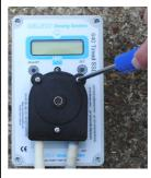
Replace the pump cover (3 thumb screws).
