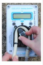
Place the tube clip in the pump head as shown. This is important. The clip should be in the housing above a mounting screw as shown.
