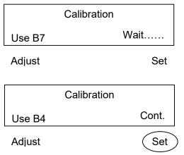
Insert the pH electrode into pH 4.0 buffer solution before pressing "Cont." The following screen will appear whilst the electrode is being calibrated against the pH 4.0 buffer solution:
