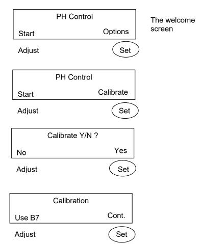
Insert the pH electrode into pH 7.0 buffer solution before pressing "Cont." The following screen will appear whilst the electrode is being calibrated against the pH 7.0 buffer solution:
