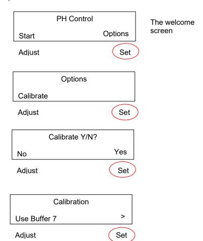
Insert the pH electrode into pH 7.0 buffer solution before pressing Set. The following screen will appear whilst the electrode is being calibrated against the pH 7.0 buffer solution:
