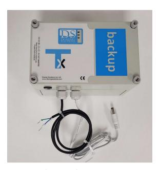
For Tx to send Alert message to warn of a power failure, it needs to have electric power to operate its modem when there is no external electric power available.
