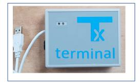
The Tx Terminal is the USB device that receives Daily Update SMS messages from any number of Tx boxes and facilitates the data contained in the messages to be stored on a computer.
