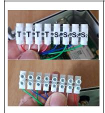
You will find connectors inside the Tx box for the temperature (T), 2 x flow sensors (F1 and F2) and the two switches S1 and S2. A small screwdriver is supplied with the Tx box to assist you.
