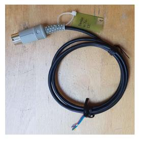
The label tag is marked "Device to Tx-I2C". There are four coloured wires inside the cable – blue, red, green, yellow. Connect the colours to any connector on the I2C board in the same positions as the colours of the connecting loom that joins the I2C board to the Tx board:
