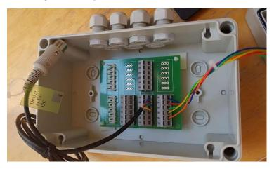
To insert the wires into the connector block, use the small screwdriver that was supplied with the Tx system to gently lever the contact jaws open:
