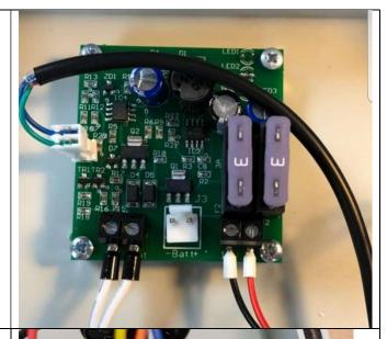
On the adapted board, a blue and green wire need to go to the Tx Switch channels. The blue is connected in with the back on the green connector as shown in the upper picture.
