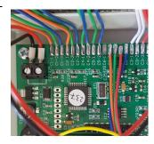
The version number of the firmware installed in each Tx box is handwritten on a paper label as shown (237 in this case).
