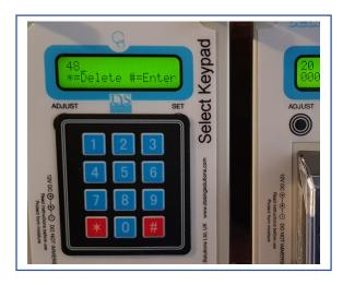
With specific programming, the Select doser will dose 960ml into the cleaning tank (48 x 20ml).
