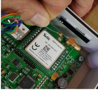
If the green light continues to flash fast, GSM signal may be low. Lift off the internal antenna connector as shown.
