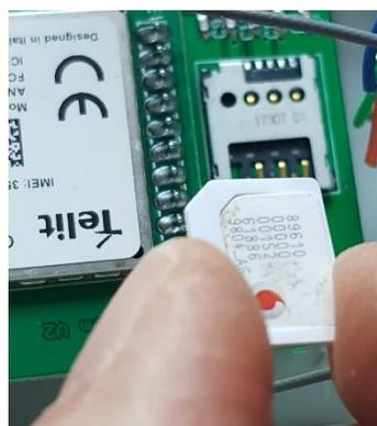
Use a Micro SIM (12mm x 15mm) and insert in the orientation shown.
