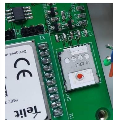
If you have large fingers, you might find it useful to temporarily remove the screw (bottom right) when installing the SIM card.
