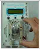
Remove the cover from the pump head.
