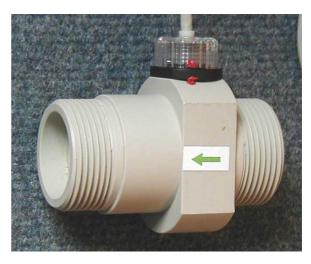
Flow range: 200 - 10,000 l/hr Flow medium:: Water only Max. medium temp.: +85 DegC Connection: 1 1/4" BSP male Pressure loss: See below
