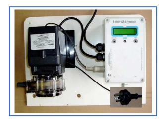
USING A peristaltic pump has the advantage that dosed products, regardless of how aggressive they are, only come into contact with the pump tube, not the working parts of the pump. Unclipping the old tube and clipping in the new one effectively cleans and renews the pump.
